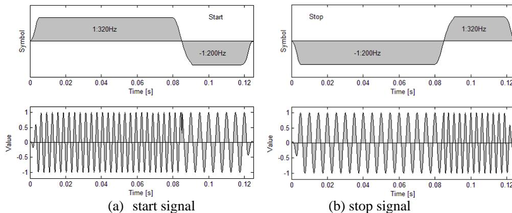
Figure 1. Two basic signals used in RoboCup.
