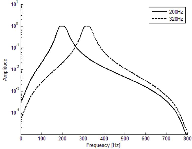
Figure 2. Frequency response of the two 4-order band-pass filters.
